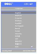
Press the  $\bigcirc$  or  $\bigcirc$  button on the control panel or the  $\triangle$  or  $\blacktriangledown$  button on the remote control to select the preferred language for the OSD.
