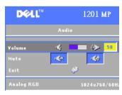
**VOLUME**—Press the ( ) button on the control panel or the - button on the remote control to decrease the volume and press the (+) button on the control panel or the + button on the remote control to increase the volume.
